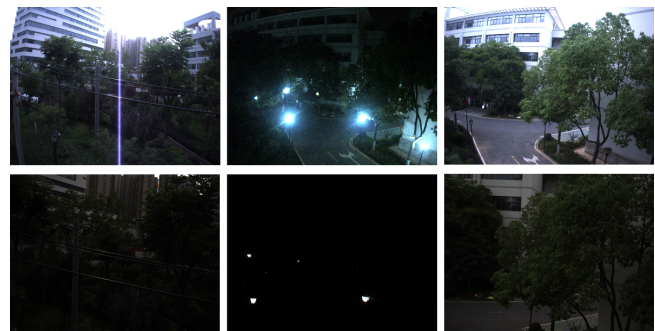
Figure 22. The different performances of the two cameras under complex lighting conditions. The upper part is the Bumblebee XB3 center camera, and the lower part is the hikvision camera. The upper and lower pairs are at the same moment.
